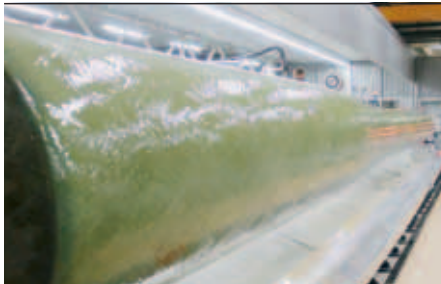
6a One-piece, filament-wound glass fiber reinforced epoxy cylinder
